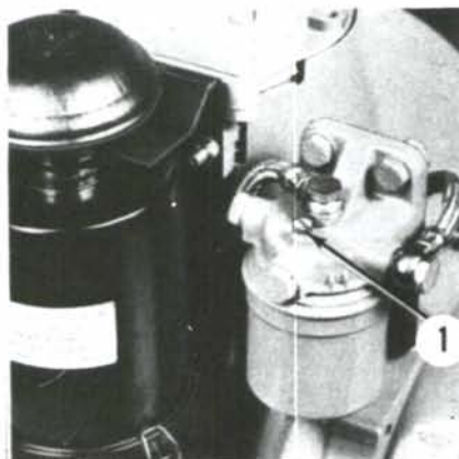
Fig. D1-1—View of air bleed screw (1) on filter housing (if so equipped).
