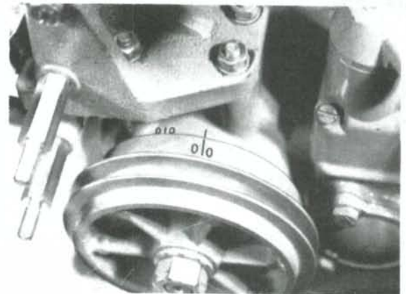
Fig. D1-4—At beginning of injection, timing marks should be aligned as shown.
